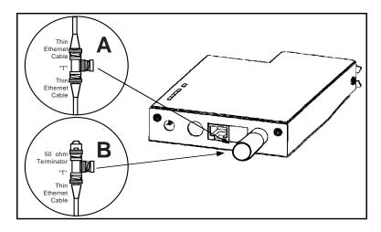
Figure 2-5 Connecting the Print Server to a 10base2 thin Ethernet network
